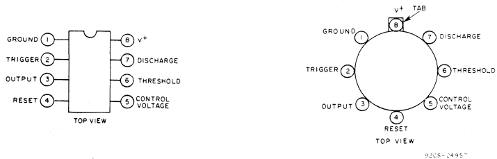
a. MINI-DIP plastic package TO-5 style package with formed leads
